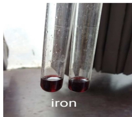
Figure 8. Test for Iron in soil sample 'a' and 'b'.
